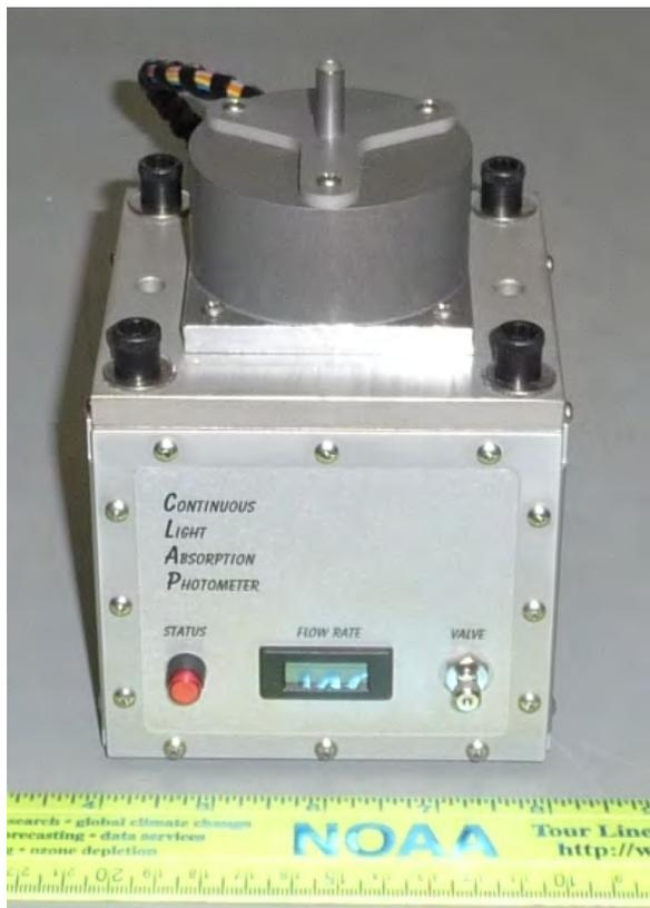
**Figure 1.** The NOAA/ESRL Continuous Light Absorption Photometer.
