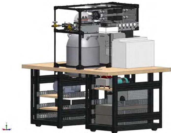
**Figure 1.** GMD’s 3-channel GC system under development. Cold-end, vacuum chamber and dewar interfaced to a thermostated chromatographic valve (VICI) enclosure. Transfer lines between the valves and the cryotrap move analytes under helium carrier flow to separation columns in the GC (Agilent 7890) and detectors (MS, FID and ECD).
