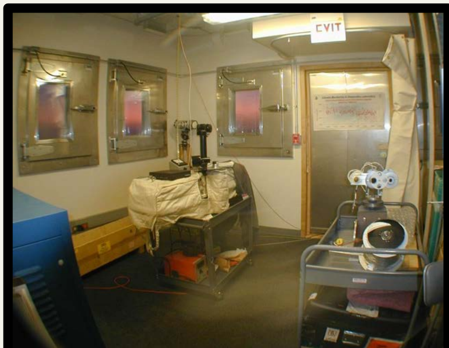
Dobson Spectrophotometer at Atmospheric Research Observatory (ARO)
