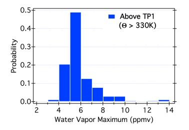
Figure 1. Histogram of the maximum summertime water vapor mixing ratios measured by the NOAA Frost Point Hygrometer above the first lapse rate tropopause (TP1) over Boulder from 1980-2014. Values exceeding 8 ppmv denote anomalously wet air masses and may indicate that convective activity significantly moistened the lowermost stratosphere.
