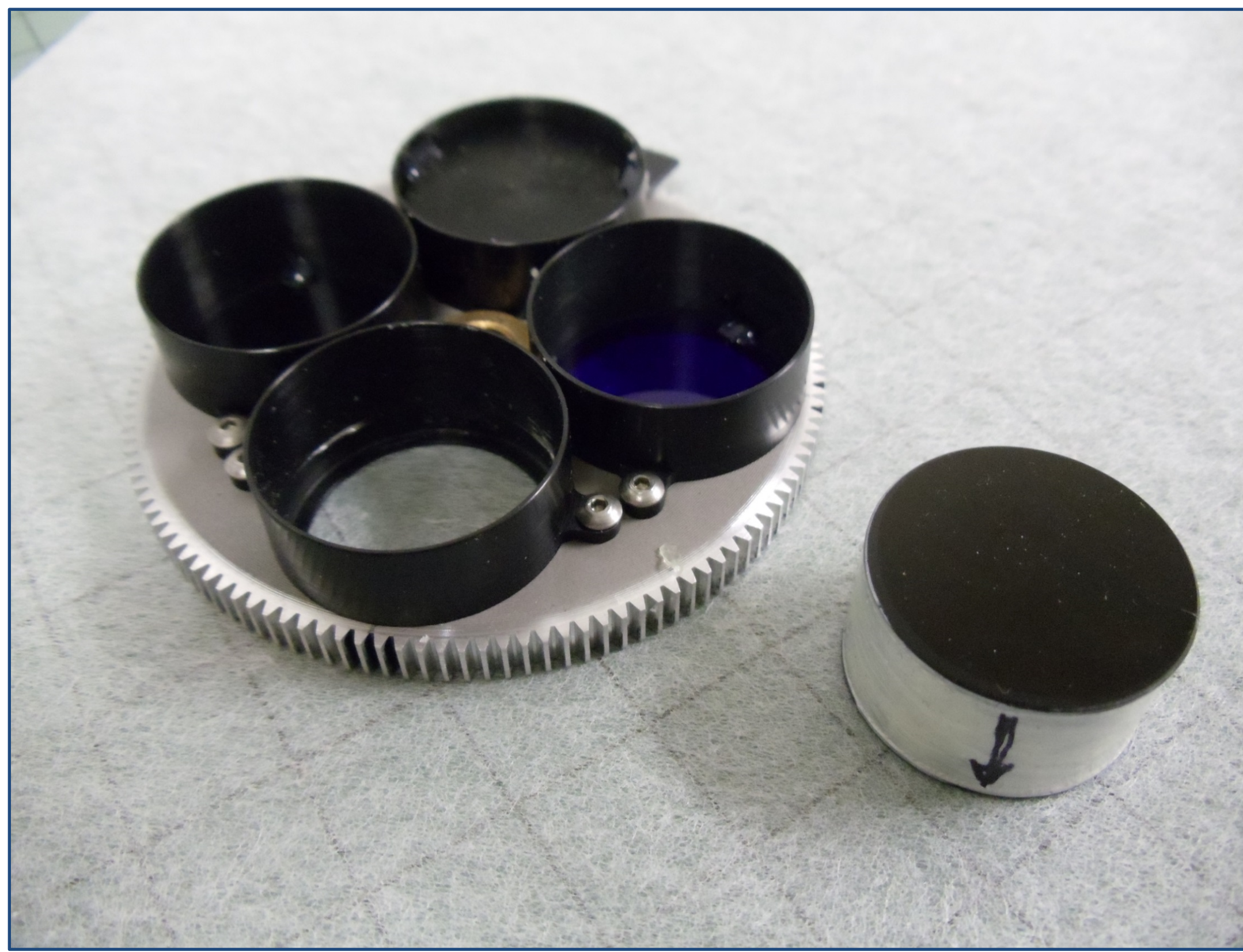
A new Inrad Optics UVC-7 combination filter ready for installation in a Brewer Mark IV spectrophotometer's filter wheel #3
