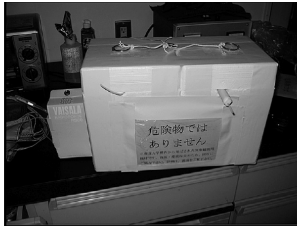
Dual ozone sonde setup as used by Morris et al., 2010. Note SO 2 filter on RH sonde.
