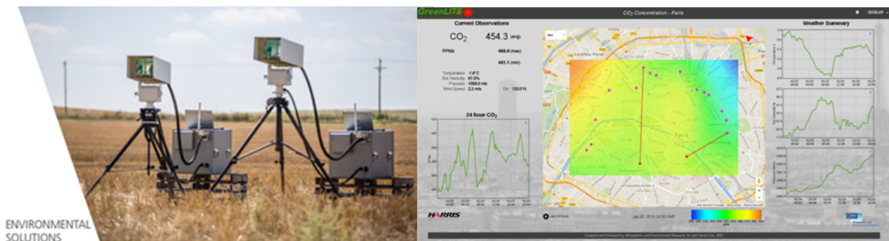
Figure 1. Prototype GreenLITE transceivers in side-by-side comparison (left), Example of the near-real time data for the GreenLITE system as deployed in Paris (right). Red dots are the transceivers and magenta dots are the reflectors. The red lines indicate the lines for a single 10 second measurement. The heat map shows the estimated concentration distribution.
