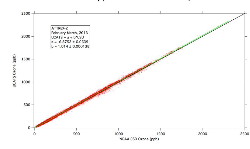
All coincident data from ATTREX-2 science flights, with merged data from the two 2B sensors in UCATS plotted against NOAA CSD ozone. Improvements to the slope came from calibrations of the pressure sensor and accounting for the pressure offset across the cell at low pressures (pressure is measured downstream of the photometer cells on the 2B sensors). Precision of the UCATS data was improved by merging the data from the two 2B
