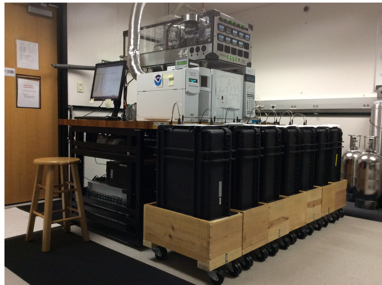
Figure 1. PERSEUS-1 (PR1) is a system for analysis of 50+ trace substances in the ambient atmosphere, using cryogenic preconcentration to increase signal to noise levels for high precision measurements. Here a full complement of seven programmable flask packages (PPFs) awaits automatic analysis. At a throughput of 65 samples per day (including standards, blanks, etc.), the twelve flasks of a PPF require ~5.5 hrs per package.
