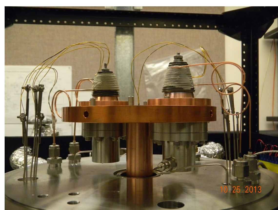
Figure 2. The cryogenic 'coldend' (patent pending) of PERSEUS allows two independent adsorbent traps to be cycled between -160°C and +100°C in under a minute for a fast analysis cycle time of 22 minutes. This device was developed with seed funds provided by a 2011 CIRES Innovative Research Proposal (IRP) to the author.
