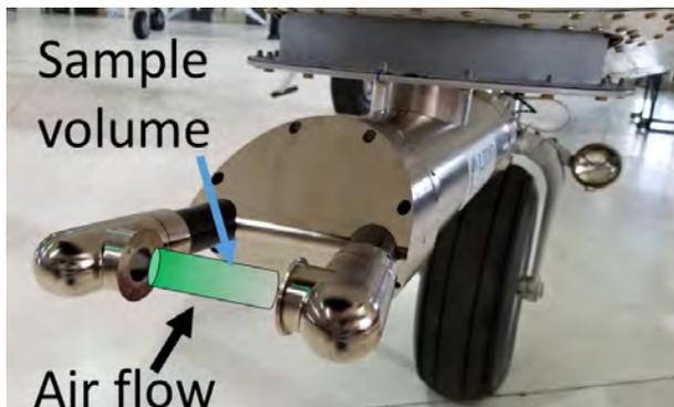
**Figure 1.** Manned aircraft version of HCPI mounted under the nose of a Twin Otter aircraft.
