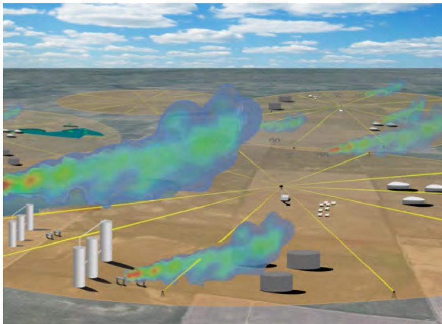
**Figure 1.** Schematic showing dual frequency comb spectrometer in the center of an observed area of potential methane sources; yellow lines show the paths of laser light beams measuring integrated open-atmosphere trace gas concentrations.
