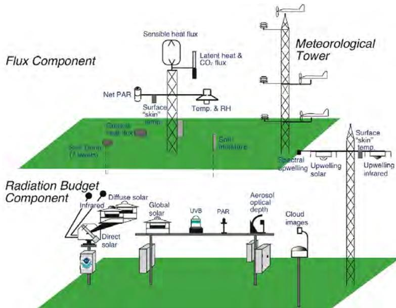
Figure 1. Details of a Prototype SEBN Station.
