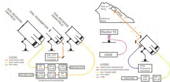
**Figure 1.** Multifrequency DIAL system consisting of a near- and far-field receiver and hybrid photon current/count detection system (left panel) and natural target IPDA system consisting of a coaxial transmitter and photon counting detection system (right panel).
