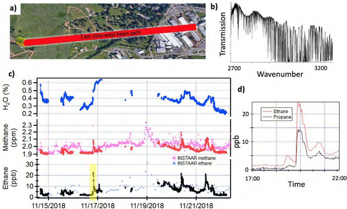
**Figure 1.** Open-path, mid-infrared, dual comb spectroscopy. (a) 1-km measurement path from NIST to Kohler Mesa. (b) Transmission spectrum showing strong water and methane absorption. (c) Retrieved path-averaged concentrations of  $\text{H}_2\text{O}$ , methane, and ethane over a one-week measurement series. The gaps are primarily due to poor weather. (d) Shorter time series showing retrieved propane.
