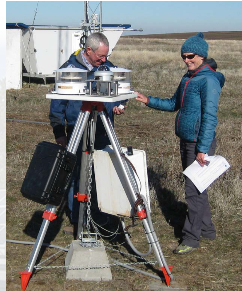
G-Rad built 3 portable radiometer systems (RADSYS) to measure spatial variability around sites
