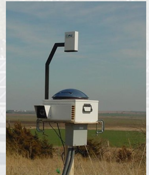
Total Sky Imager measures fractional sky cover (cloud fraction)
