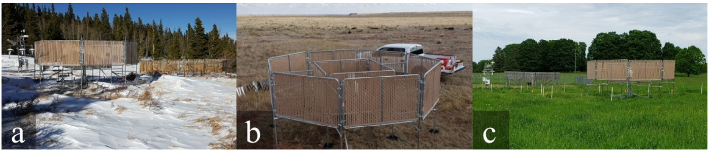
Figure 1. Photos of Low Porosity Double Fence (LPDF) shields installed at the Boulder, CO (a), Marshall, CO (b), and Chatham, MI (c) sites.
