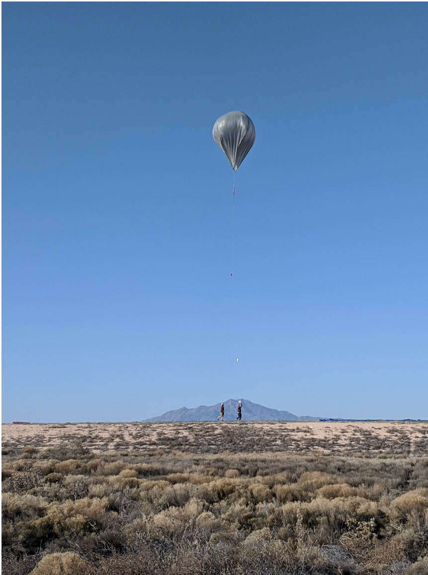
Figure 1. Launch of a solar balloon from Belen, New Mexico, carrying atmospheric sensors for temperature, pressure, and aerosols.
