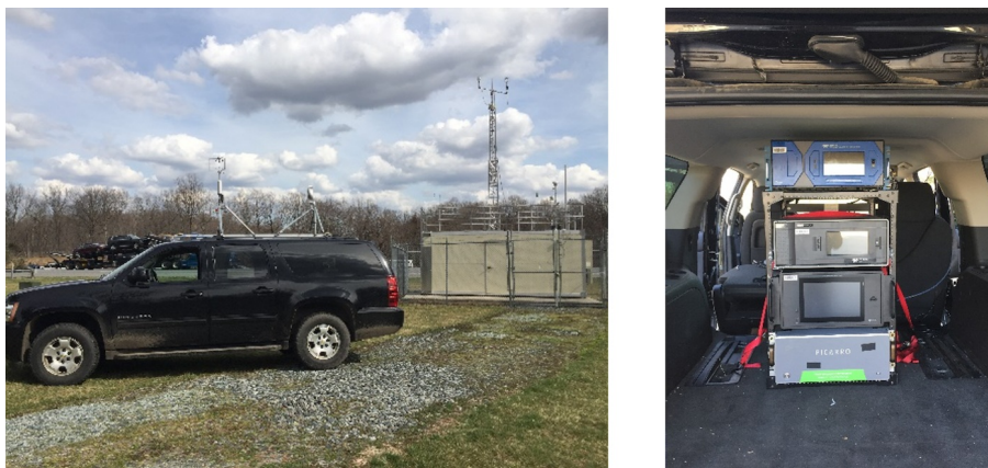
Figure 1. Left: The mobile van parked next to a near-road air quality monitoring site with instruments running. Right: Some instruments inside the mobile van.
