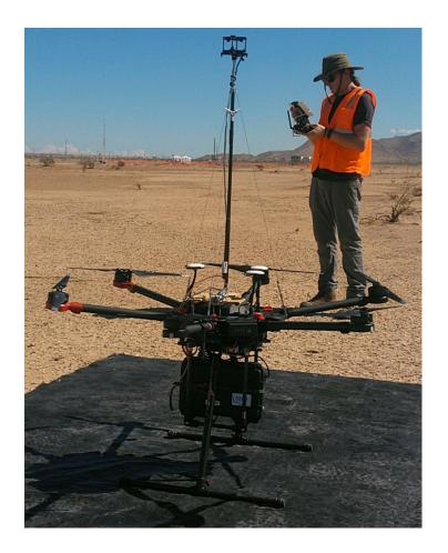
**Figure 1.** Pre-flight preparations of unmanned aerial system for direct methane flux mesurements.
