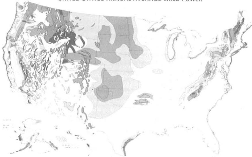
Figure 1.--Wind energy in the United States. (Map courtesy of Battelle, Pacific Northwest Laboratories.) Darkest shading indicates greatest wind energy.
