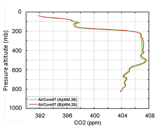
Fig. 4-8: Vertical profiles of CO<sub>2</sub> in two different AirCores flown simultaneously to an altitude of 28 km.
