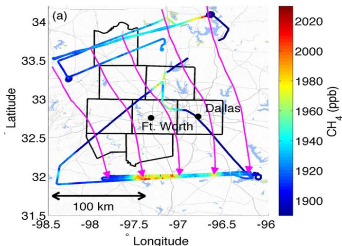
Fig. 4-5: Flight pattern on 19 October 2013 over the Barnett Shale oil and gas field for “mass balance” estimation of total methane leaks from the area. The downwind enhancement of the  $\text{CH}_4$  mole fraction and the wind speed and direction (pink arrows from northwest veering toward south), as well as the boundary layer height are used. There were multiple transects downwind at different altitudes.
