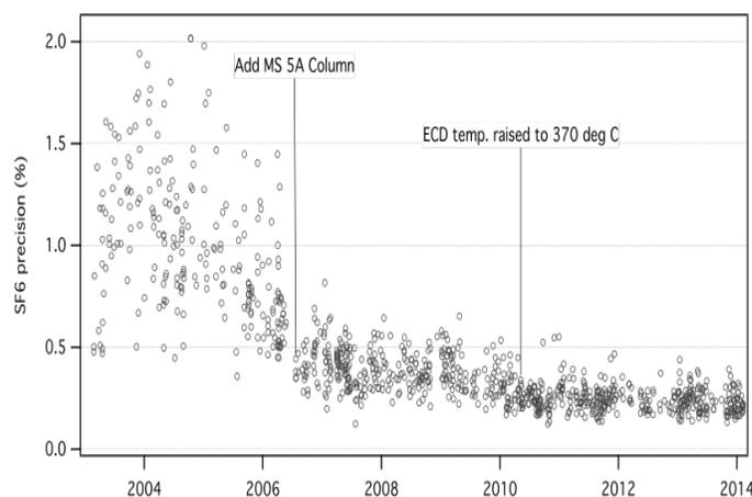
Fig. 8-1: Analytical precision (%) of SF<sub>6</sub> calibration measurements since 2003 for SF<sub>6</sub> mole fractions in the range 4–12 ppt. Note the improvement in precision in 2006 corresponding to the addition of the molecular sieve 5A column.
