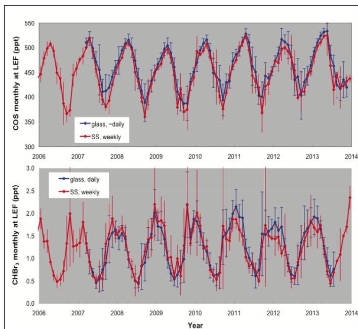
Fig. 5-5: Monthly mean mixing ratios for carbonyl sulfide (COS) and bromoform (CHBr<sub>3</sub>) at LEF as determined from two different instruments, flask sampling apparatus, and flask types. Results from M2 (blue line) are from 10 to 50 glass flasks sampled per month with the automated CCGG programmable compressor package; results from M1&M3 (red line) are derived from paired SS flasks sampled once per week. Error bars represent one standard deviation of the results obtained during each month.
