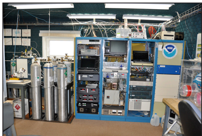
Figure 2.3: Barrow Observatory instrument racks with CO 2 , meteorology and the station data networking system controllers.
