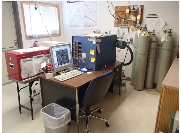
Figure 2.9: Mauna Loa Observatory halocarbon gas chromatograph and calibration gas tanks in a room maintained at a constant temperature.
