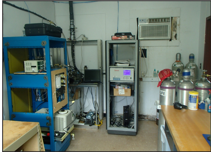
Figure 2.13: Inside the American Samoa Observatory Hudson Building with Scripps instruments including surface ozone and gas calibration tanks.
