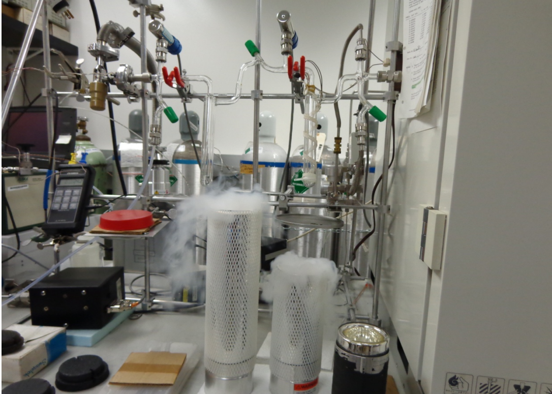
Glass manifold on the CO 2 manometer used for extracting CO 2 from air. The manometer is used to determine the mole fraction of CO 2 on an absolute basis.
