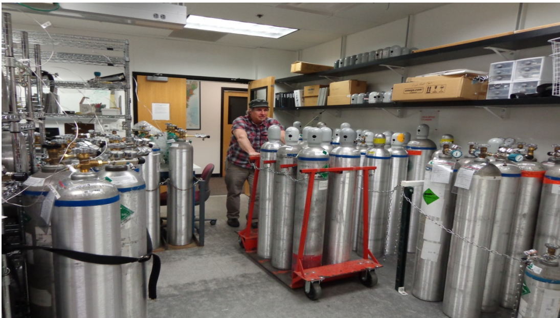
Moving gas cylinders into the CO 2 calibration laboratory. Here, CO 2 mole fractions are assigned based on the WMO X2007 scale.
