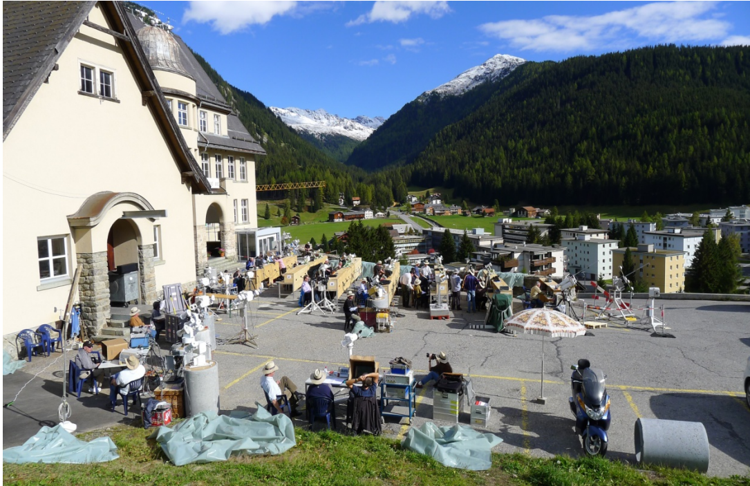
International pyrheliometer comparison Davos, Switzerland, 2010. GMD scientists are testing GMD instruments against the World Radiometric References.
