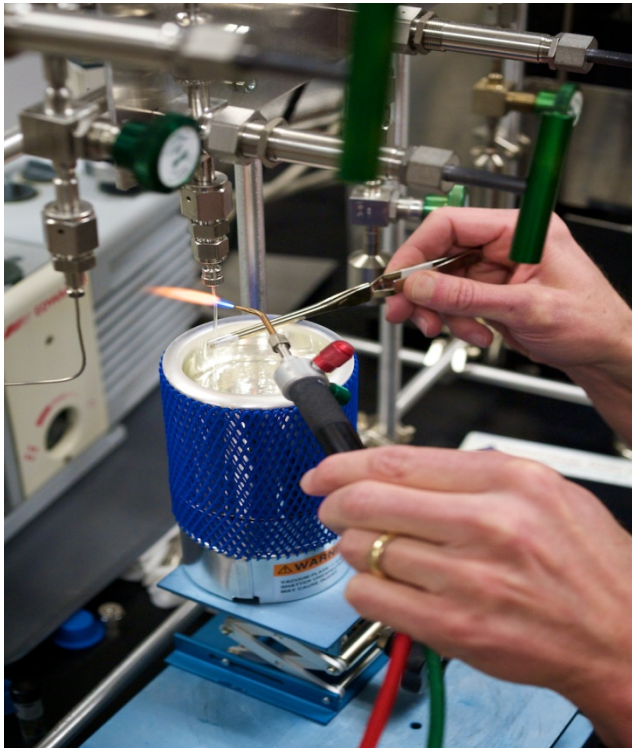
A step in preparing a gas standard by sealing a known amount of a specific gas into a glass capillary tube. The gas will later be added to a large tank of air to produce a standard.
