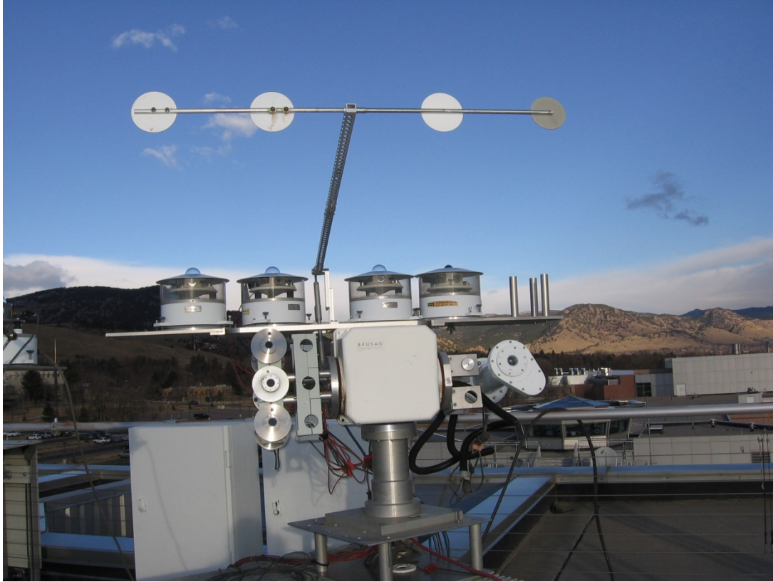
Diffuse and direct solar radiation instrument calibrations at the GMD Boulder, Colorado rooftop facility.
