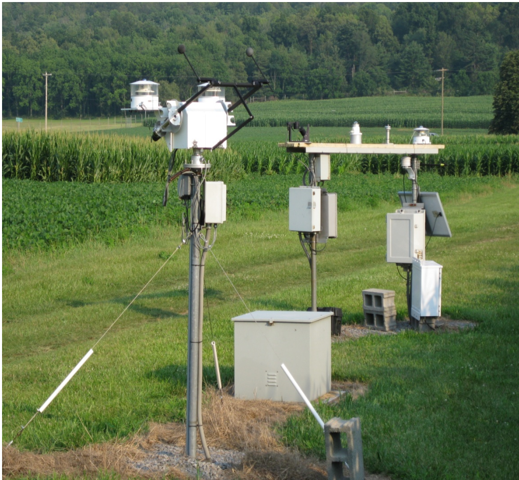
GMD Surface Radiation (SURFRAD) network site at Pennsylvania State University near State College, PA. The data from this and 6 other SURFRAD sites distributed across the U.S. are transmitted daily to GMD, Boulder.
