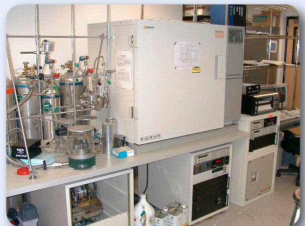
Natural-air gas standards are prepared in the Rocky Mountains, near Boulder. Over 500 compressed gas cylinders were filled, calibrated, and distributed world-wide in 2012.
